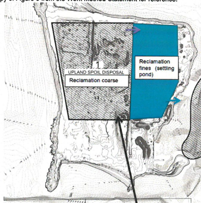
Figure 5 – Typical distribution of reclamation area and flow of mixture
