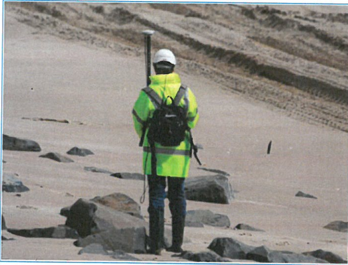
Figure 18 - Typical manual topographic GPS survey
