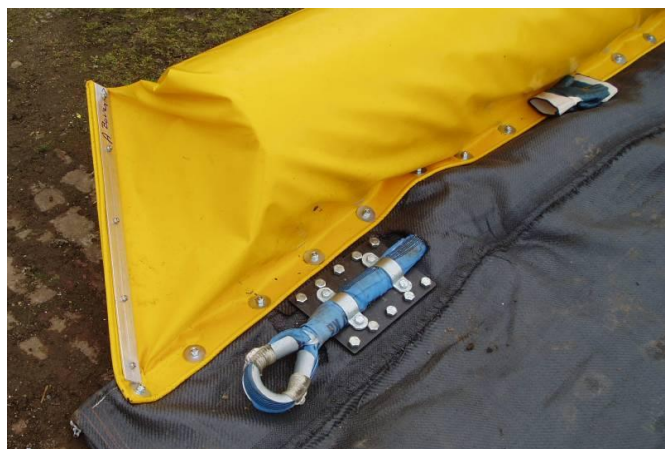
Figure 6 – "Geolon silt screen" with bolted connection to the Styrofoam float
