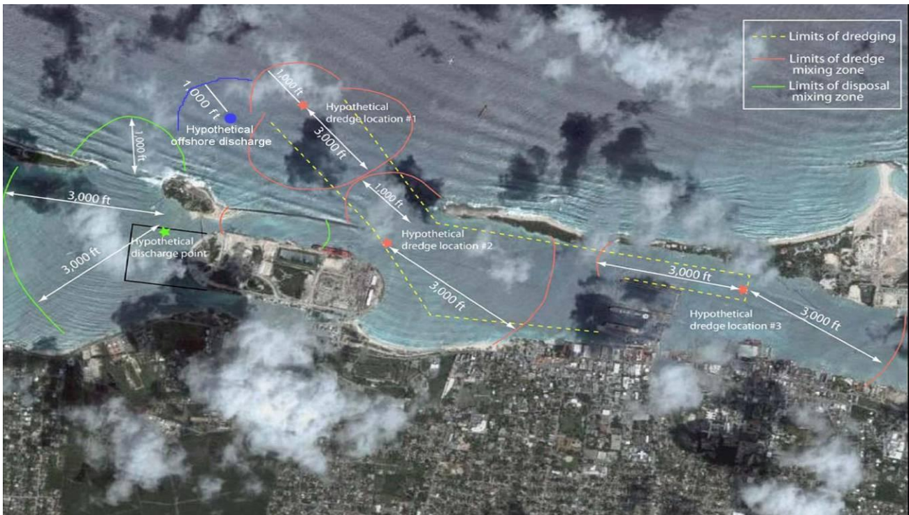
Figure 10 - Turbidity Mixing Zones for various dredging and discharge locations. Current runs west to east.
