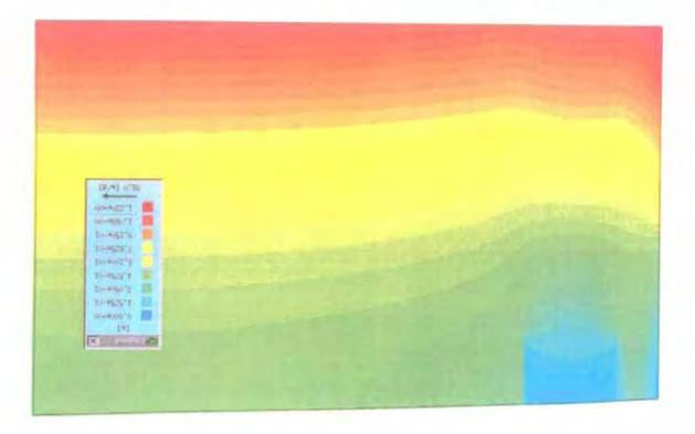
Figure 23: Distribution of heads in m (Albany Marins and curtainwall, fringes in segment 1, vertical exaggeration 20x)
