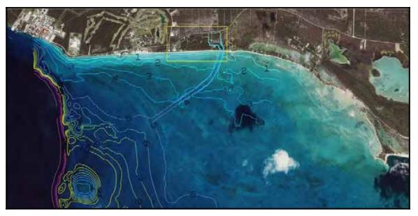
Figure 5.2 Alignment of marina access channel
