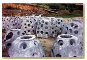
Figure 7: Reef Balls: hollow concrete domes are produced to eventually be towed and placed on the ocean floor to enhance coral and fish habitat
