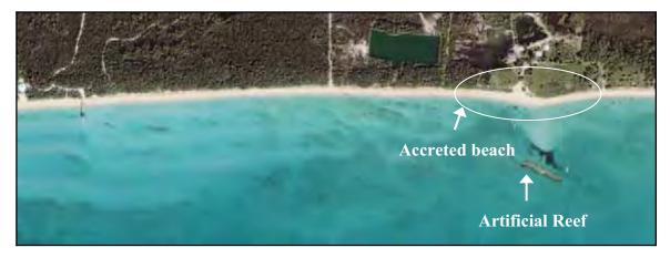
Figure 1: Artificial Reefs and Sandbars in the nearshore zone, Albany Development
